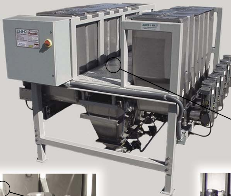
Center walk aisle, constructed from Carbon Steel Checker Plate with Kick-rail
