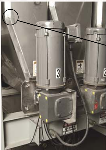
Interior 45 degree corners to improve product flow and reduce bridging
